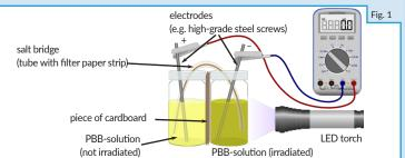
Following figure 1, set up the experiment and switch on the LED torch. Observe voltage and colour for three minutes. Switch off the light and observe another three minutes. Name all forms of energy which are involved in the experiment.
